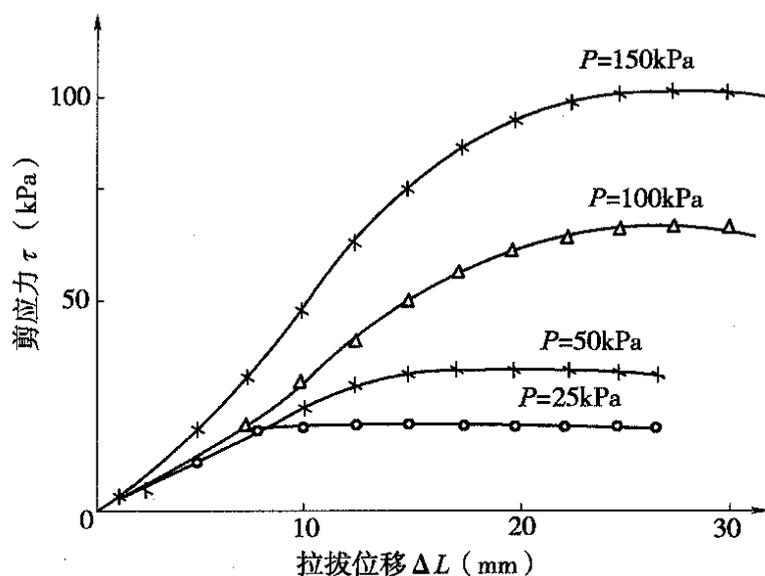
图 T 1130-2  $\tau$ - $\Delta L$  曲线
